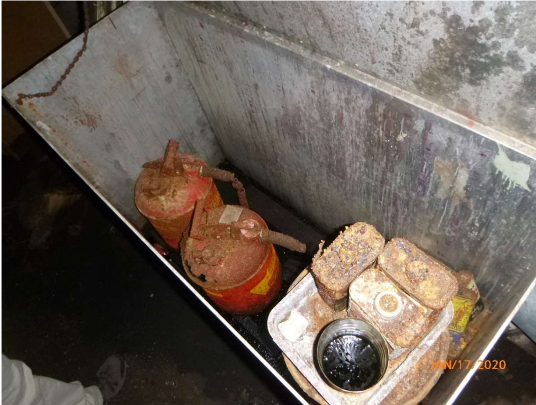
Photo 27. Storage bin containing fuel (kerosene) and solvents with residue in the bottom.
