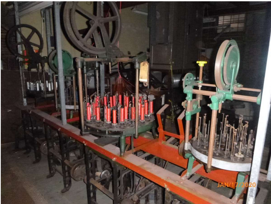
Photo 24. Manufacturing equipment that uses multiple spools to braid thread together.
